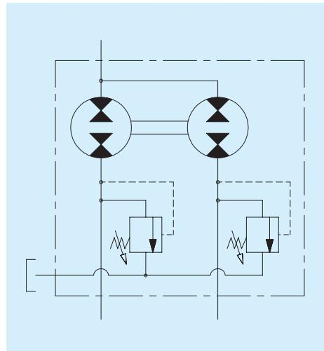
**VE** With adjustable pressure relief valves and single inlet on the cover
