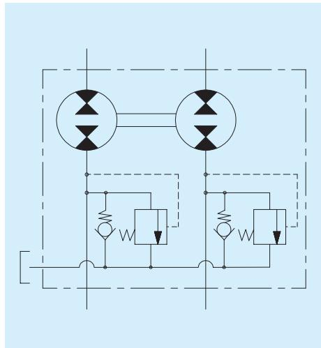
**VC** With fixed pressure relief valves and single inlet on the body
