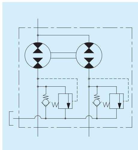
**VC** With fixed pressure relief valves and single inlet on the cover
