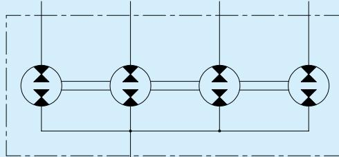
The flow dividers in groups 1 and 2 can be supplied with pressure relief valves to allow rephasing of the actuators at the end of the stroke. The valves can be calibrated and positioned on each section of the divider whereas the
