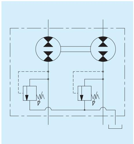
**VE** With adjustable pressure relief valves and single inlet on the body
