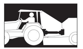
When used at night or in poor visibility, illuminate the driveline operating area.
