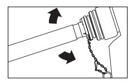
Attach the shield restraint chains, allowing sufficient slack for the driveline to move during turns and operation.
