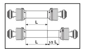
Keep the profile tubes overlapped as much as possible during transport and operation. Do not exceed the values given in this catalog for permissible length extension. If greater telescoping ability is required, contact Bondioli & Pavesi engineering.
