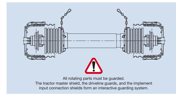
Proper use and maintenance of the driveline and shielding is of primary importance for operator safety.
