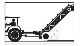
Always hitch the tractor to STATIONARY MACHINERY (pumps, hoists, generators, dryers, etc.). Check the tractor wheels to prevent rolling and check that joint angles are small and as equal as possible.
