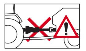
Ensure that all driveline, tractor, and implement shields are functional and in place before operation. Damaged or missing parts must be replaced with the original equipment spare parts, correctly installed, before using the driveline.
