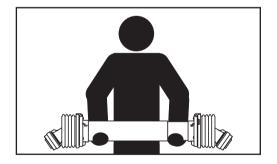
Keep the driveline horizontal during handling to prevent the halves from sliding apart, which could cause injury or damage the shielding. Use suitable means to transport the driveline, depending on the weight.
