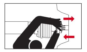
Ensure that the driveline is securely attached to the tractor and the implement before operating. Check that all bolts or nuts are properly torqued.
