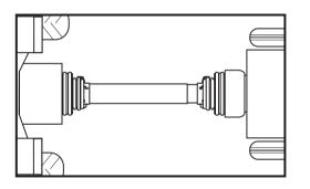
All rotating parts must be guarded. Contact with a rotating driveline can cause death or serious injury. The tractor master shield, the driveline guards, and the implement input connection shield form an interactive guarding system.
