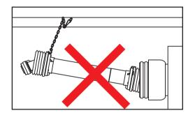
Never use the shield restraint chains to support the driveline for storage. Always use the support on the implement.
