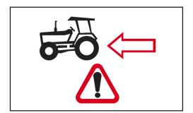
The tractor printed on the shield indicates the tractor end of the driveline. Any torque limiter or overrunning clutch must be installed on the implement end of the driveline.
