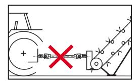
Always hitch the tractor to STATIONARY MACHINERY (pumps, hoists, generators, dryers, etc.) so that the profile tubes are not overextended. Under all working conditions, extension of the driveline should not exceed the values reported in this catalog. All rotating parts must be guarded.
