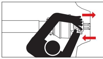
Ensure that the driveline is securely attached to the tractor and the implement before operating. Check that all bolts or nuts are properly torqued.
