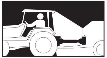
When used at night or in poor visibility, illuminate the driveline operating area.
