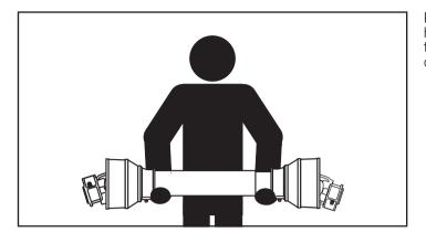
Keep the driveline horizontal during handling to prevent the halves from sliding apart, which could cause injury or damage the shielding. Use suitable means to transport the driveline, depending on the weight.
