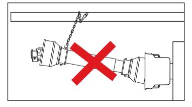
Never use the shield restraint chains to support the driveline for storage. Always use the support on the implement.
