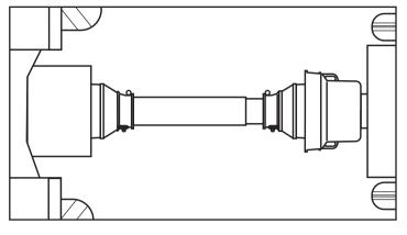
All rotating parts must be guarded. Contact with a rotating driveline can cause death or serious injury. The tractor master shield, the driveline guards, and the implement input connection shield form an interactive guarding system.
