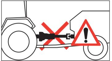
Ensure that all driveline, tractor, and implement shields are functional and in place before operation. Damaged or missing parts must be replaced with the original equipment spare parts, correctly installed, before using the driveline.
