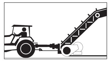
Always hitch the tractor to STATIONARY MACHINERY (pumps, hoists, generators, dryers, etc.). Chock the tractor wheels to prevent rolling and check that joint angles are small and as equal as possible.
