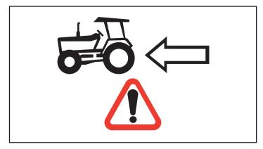
The tractor printed on the shield indicates the tractor end of the driveline.
