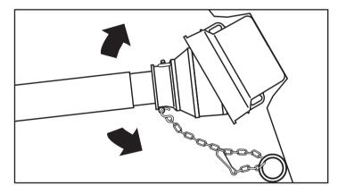
Attach the shield restraint chains, allowing sufficient slack for the driveline to move during turns and operation.
