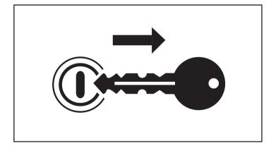
Disengage the PTO, turn off the tractor engine, remove the key, and check that all rotating parts have come to a standstill before approaching the implement or performing maintenance work.
