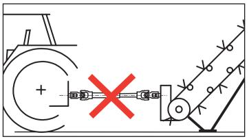
Always hitch the tractor to STATIONARY MACHINERY (pumps, hoists, generators, dryers, etc.) so that the profile tubes are not overextended.
