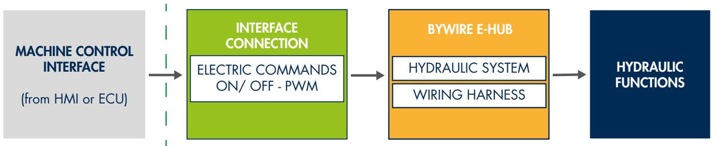
ByWire HUB is an integrated system for the control and management of ByWire valves by a single connector. ByWire HUB is available in three versions.
