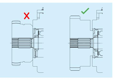
Measure the distance on the motor between the outer surface of the bell and the end of the teeth of the flange mounted on the flywheel. Measure the distance between the surface of the pump flange and the end of the hub teeth
