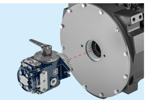
Position the pump to align the centres of the screw slots\* with the threaded holes on the bell.
