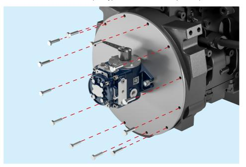
Secure the bell with screws (the type of screw is not important).
