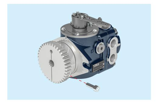
For gear pumps with a European flange and conical shaft (Gr. 2 and Gr. 3), first fit the adapter ring and then the hub in the pump centring, sliding it to the end of its stroke. Lastly, secure it with the nut on the head of the shaft itself.
