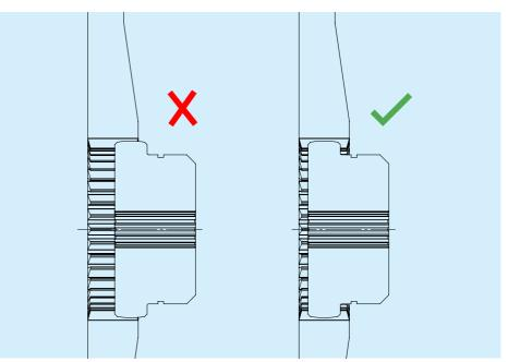
Tighten the hub on the pump shaft by screwing the screw provided to the tightening torque shown in the following tables for KVS or KDR versions:
