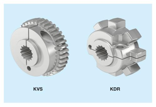
For grooved shafts, fit the KVS or KDR hub on the pump shaft, maintaining the mounting measurement indicated by HP on the drawing. If this measurement is not indicated, slide the component until it is snug on the shaft.
