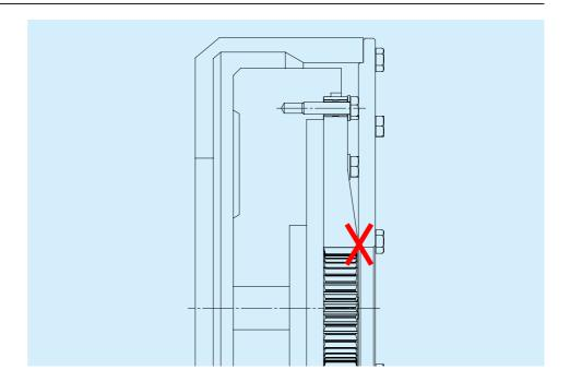
Secure the bell using screws\* as preferred (screw type is not important).
