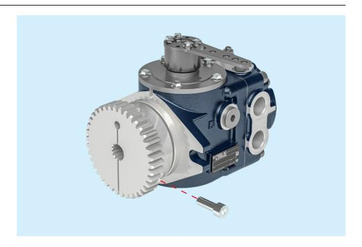
For gear pumps with a European flange and conical shaft (Gr. 2 and Gr. 3), first fit the adapter ring and then the hub in the pump centring, sliding it to the end of its stroke. Lastly, secure it with the nut on the head of the shaft itself.
