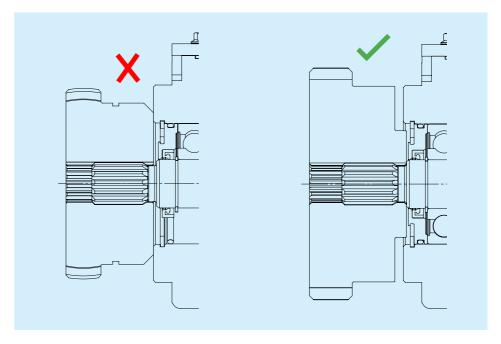
Measure the distance on the motor between the outer surface of the bell and the end of the teeth of the flange mounted on the flywheel. Measure the distance between the surface of the pump flange and the end
