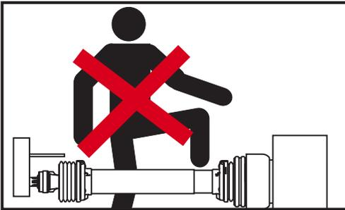
Do not stand, lean, or otherwise come in contact with the driveline. Do not step over or go under the driveline.
