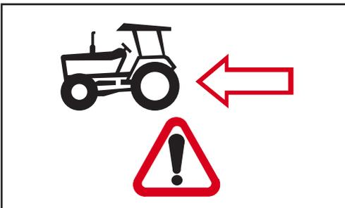
The tractor printed on the shield indicates the tractor end of the driveline. Any torque limiter or overrunning clutch must be installed on the implement end of the driveline.
